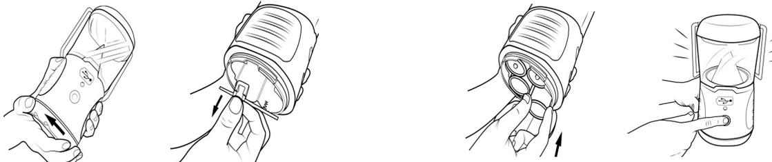
1. Remove base of the Lantern by rotating clockwise.
