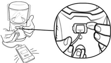
5. To charge a device, open USB Port Cover. Plug your device's USB cord into USB Port.
