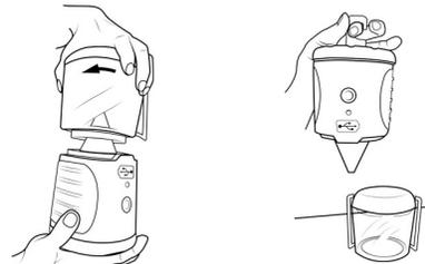
7. Remove top of the Lantern by rotating lid clockwise and pulling apart.
