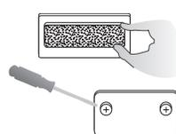
7. Mount Bracket to wall with double sided tape, holding for 10 seconds or install with 2 small screws.
