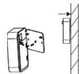
8. Slide light onto mounting bracket attached to wall.
