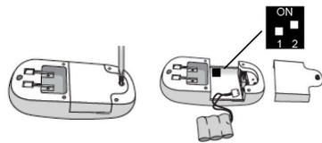
1. Loosen the screw and remove the battery door on the MB220.
