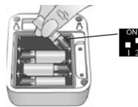
3. Insert 4 new Alkaline AA Batteries, with correct polarity/position.
