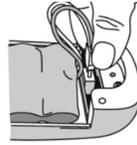
3. Plug battery into flashlight with red wire on the left and close battery lid. Secure screw.
